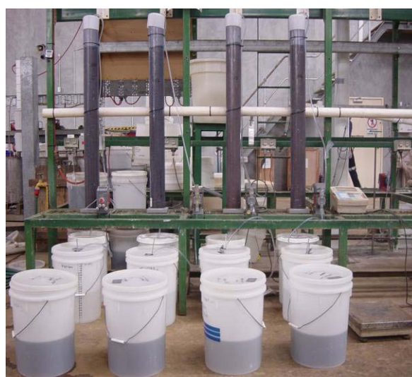
Photo: Four sample columns containing the agglomerated laterite with the buckets containing the leachate solution.
