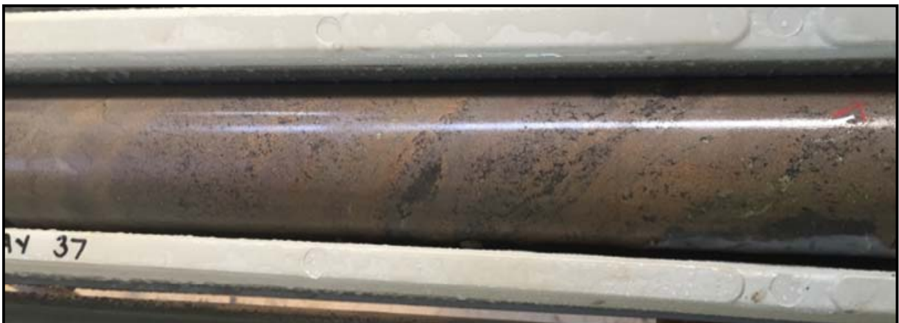
Figure 3: Massive sphalerite rich drill core intersection from WNDD0138 in the G2 Hanging Wall position. Handheld Niton XRF analysis of these sphalerite rich massive sulphide zones returned an average of approximately 30% Zn (some 25 readings taken) over the interval 120.4 to 126.4m. The average zinc grade, however, is expected to be slightly lower than this as the handheld XRF reading does not take into account some internal gangue and other dilution. The interval shown here is approximately 80cm long.
