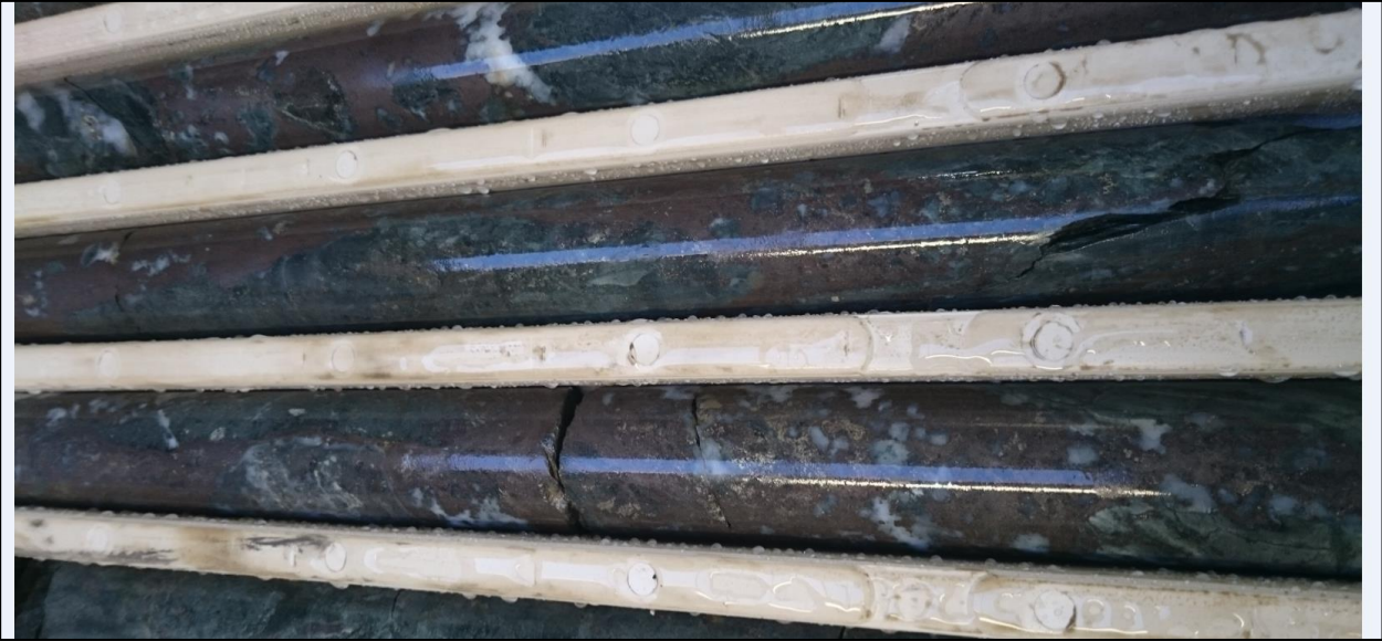
Figure 2: Photo of the zinc sulphide (sphalerite stringers) in CWDD0001 from 486m. NQ2 (46.7mm) core within the core tray with each length approximately 1m long.
