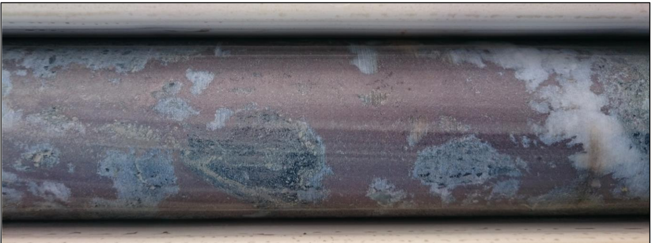
Figure 3: Drill core detail showing massive zinc sulphides. The red-brown mineral is sphalerite (zinc sulphide) and shows a hydrothermal, replacement style of formation with clots of dark green chlorite being original basalt fragments entrained within the sphalerite. The white mineral is quartz and indicates the vein-style of formation of this zone.
